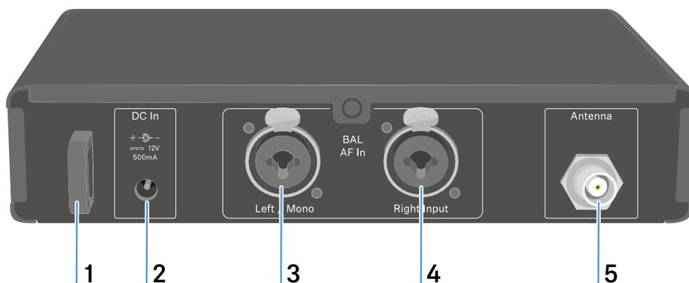
**1** Strain relief for the connection cable of the power supply unit
