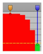
When you click on a marker, the line and the flag turn to orange. When you move the mouse pointer over a marker, a box will appear above the marker, indicating the time and the measured field strength of both antennas.
