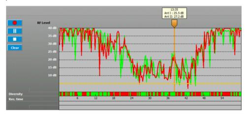
The measured values of the field strength "RF Level" are displayed as colored bars over the defined measuring duration. Field strength levels of up to 40 dB max. can be displayed.
