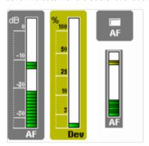
The threshold values are displayed in color in the modulation display. A yellow section in the bar graph indicates that the transmitter is fully modulated. An additional red section indicates overmodulation. If this occurs, reduce the modulation level on the transmitter.
