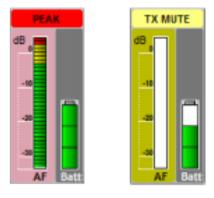
The messages are highlighted in different colors. The part of the panel to which the message refers is also highlighted.
