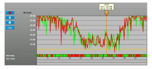
The measured values of the field strength "RF Level" are displayed as colored bars over the defined measuring duration. Field strength levels of up to 40 dB max. can be displayed.
