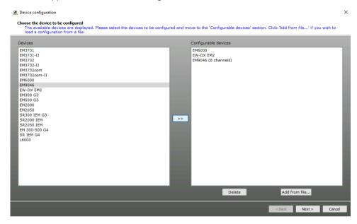
The window contains two lists. The left-hand list displays all WSM compatible devices. The right-hand list displays your current device selection.
