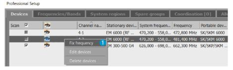
→ If the frequency of a device is fixed, a lock icon appears next to the frequency of the device 2.
