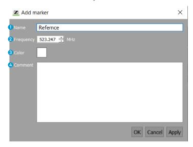
After confirming the "Add marker" window by clicking on "OK", the marker 1 is displayed in the upper window area of the "Markers" tab.
