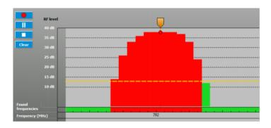
This window displays the measured field strength of the different frequencies within the receiver's frequency range as vertical bars (display range of up to 40 dB).
