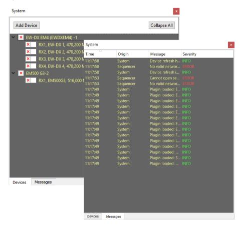
With the standard settings, the display area 3 is divided in two. The "panels" for the connected devices are displayed on the left; this region is designated as the scene.
