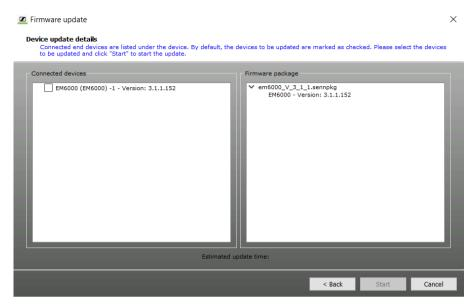
The "Firmware package" box on the right displays all available firmware versions from the selected SENNPKG file. The "Connected devices" box on the left displays the corresponding connected devices.
