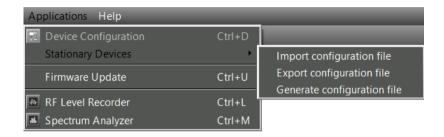
The "Stationary Devices" menu item in the "Application" menu allows you to define, add and export new frequency ranges for existing stationary devices.
