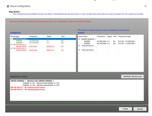
The left-hand list displays the pre-configured devices ("Offline Configuration"). The right-hand list displays all currently connected devices. The device assignment appears in the "Comparison result" window.
