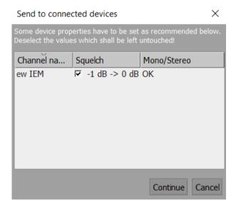
The recommended squelch levels are sent to the corresponding devices together with the allocated frequencies.
