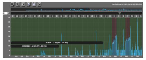
Usable frequency ranges are displayed in transparent green (can be viewed/hidden via the "Usable bands" check box in the "Freq./band filters" area.
