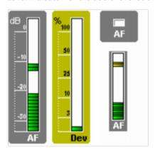
The threshold values are displayed in color in the modulation display. A yellow section in the bar graph indicates that the transmitter is fully modulated. An additional red section indicates overmodulation. If this occurs, reduce the modulation level on the transmitter.
