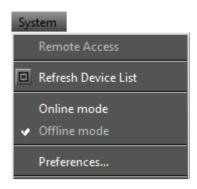
**Remote Access:** Activates or deactivates access to the parameter settings of the devices (see Displaying an overview of parameters).
