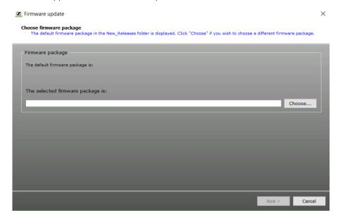
If there is a new firmware version available in the "New Releases" folder of the program folder, it is displayed in the "The selected firmware package is:" field.
