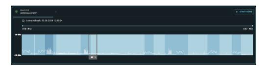
Before activating the connected antenna, you can check the occupancy of the frequency spectrum and examine the surroundings for possible frequency interference.
