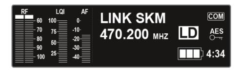
In the displays, the home screens for both channels display the **channel-specific status information** such as the reception quality, battery life, audio level, and so on. See Home screen.
