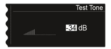
i While the test tone is played back, the transmitter audio signal is muted.
