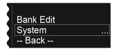
On the display for the channel CH 1, the system settings for the whole device are also displayed in the operating menu. See System menu item.
